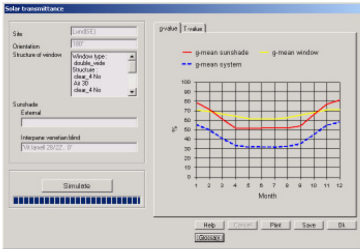
Figure 6.12.b Monthly mean g-values of the interpane sunshade “White slat 28/22”, 0° slat angle, from ParaSol simulations.
