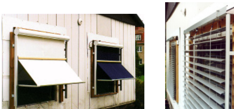
Figure 2.1 Twin-boxes equipped with Italian awnings (left), and external venetian blinds (right).
